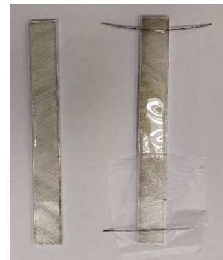
Figure 3: Making an adhesive joint
